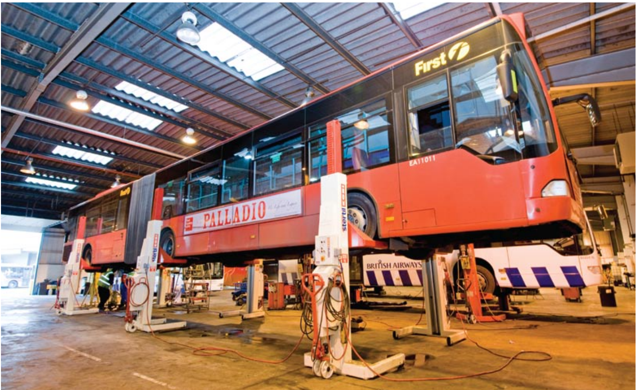
Figure 48 Six-synchronised mobile lifts
