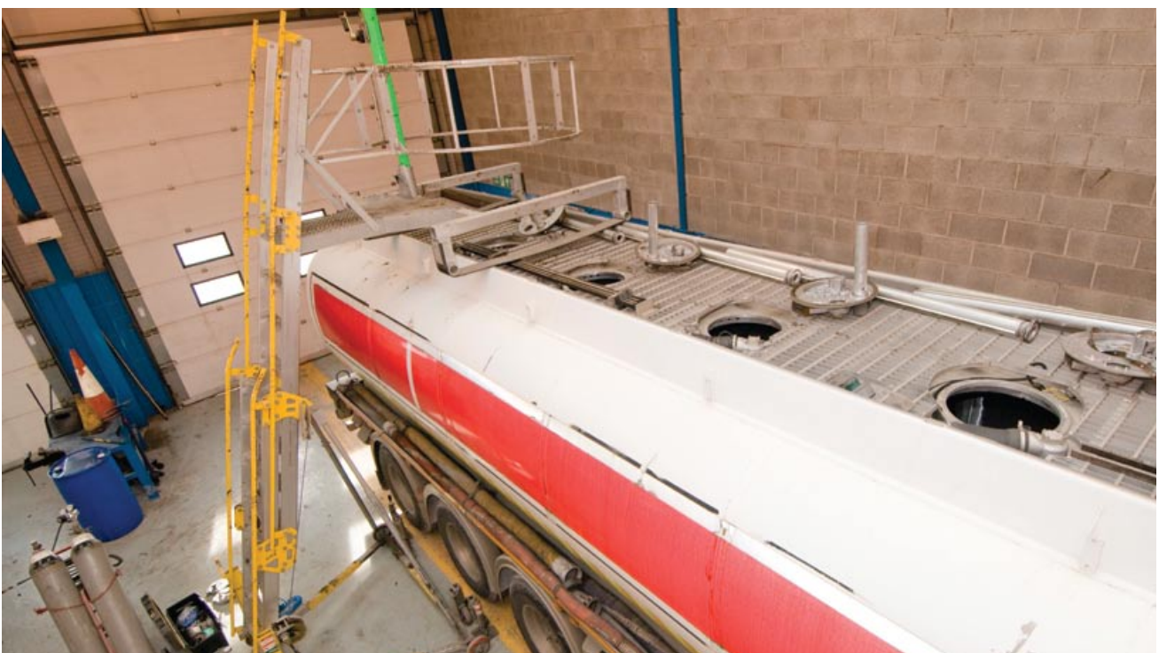
Figure 83 Ladder access and harness provision for working on top of a tanker
