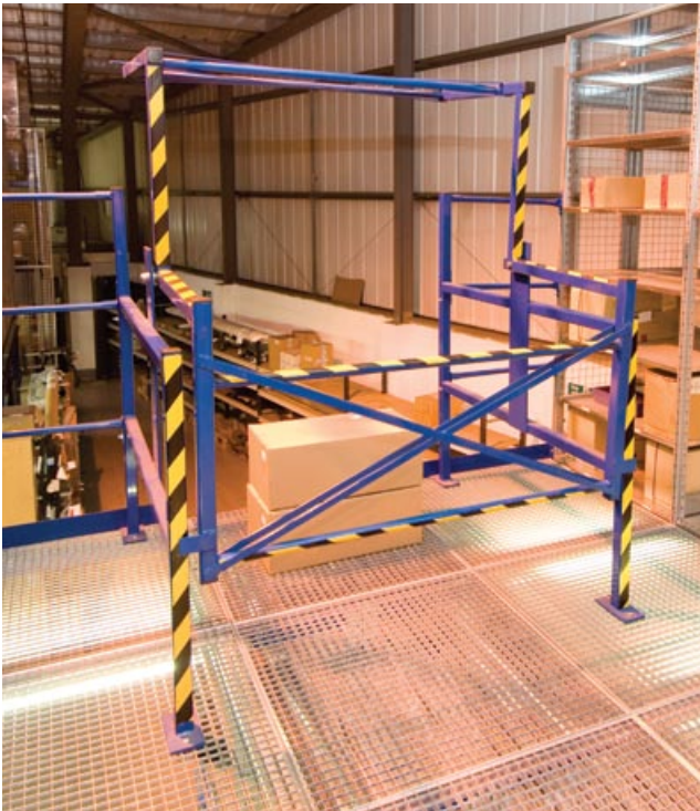
Figures 88 and 89 Pivoting safety barrier ensures that the fence opening is guarded at all times
